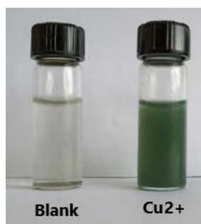
Fig.1: Colorimetric response of chemosensor in the presence of \text{Cu}^{2+} ; color changes in aqueous solution (100 ppm) at pH = 5.5.
