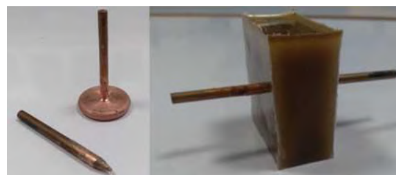
Fig.1: Electrodes and the prepared sample fore dielectric breakdown strength test
