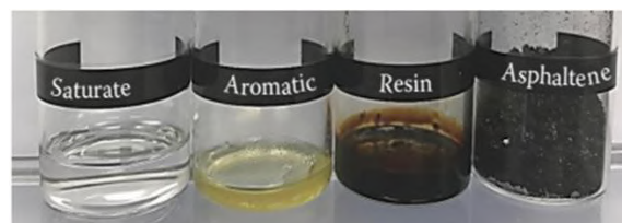
Fig.2: SARA separation for a crude oil sample [5].
