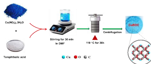
Fig.1: Preparation of Cu-BDC using hydrothermal method
